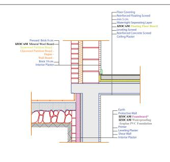
\* Should not be adhered with hot asphalt.
