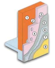
Exterior wall ① Fixing mortar ② Plastic anchor ③ Manto Foamboard ④ Undercoat plaster ⑤ Plaster loading mesh ⑥ Undercoat plaster ⑦
